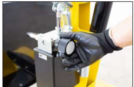
Detail of the hand pump with rod housing support and knurled knob
